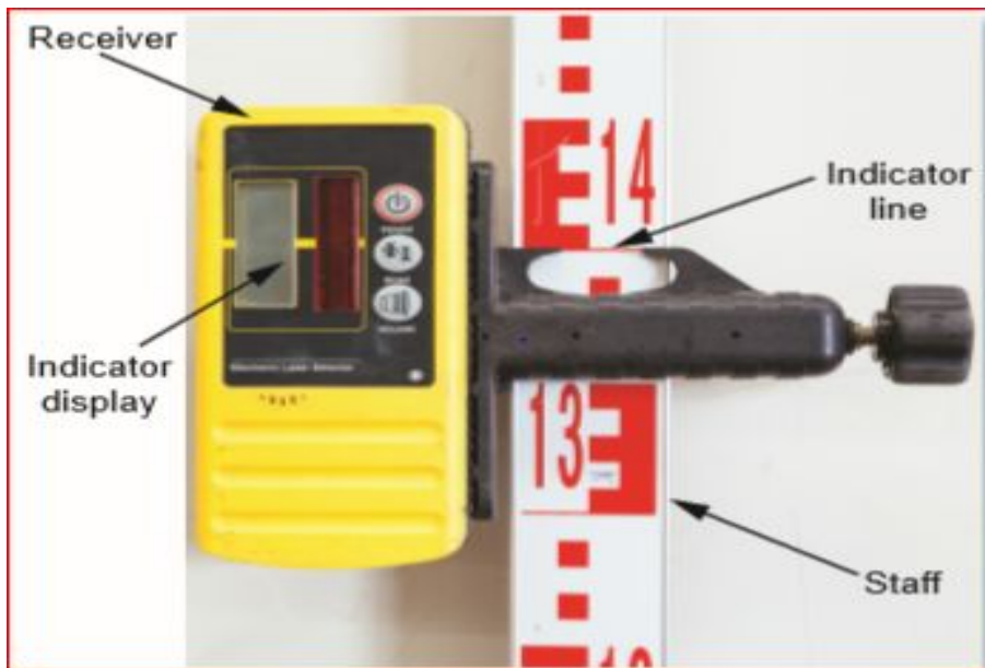
Figure 6 locking receiver on the staff
