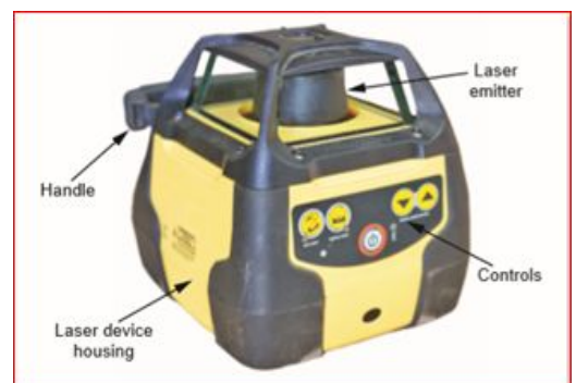
Figure 21 parts of Laser level
